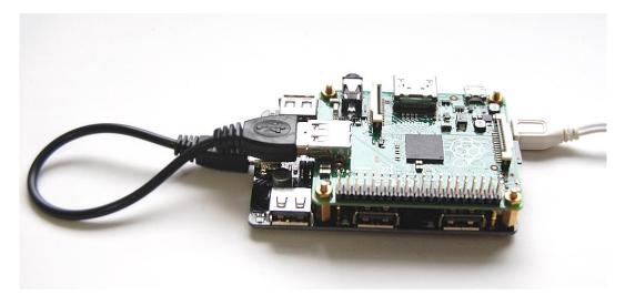
Different than the B+ model, Raspberry Pi A+ supports back-powering via USB port. So it is not necessary to use those pogo pins for back-powering. Just make sure to place the jumper to "power link" position and only connect a power supply to the USB hub, then Raspberry Pi A+ can be back-powered by the USB hub.
