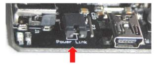
If you don't want the back-powering, just put the jumper to the other side and connect two power supplies to USB hub and Raspberry Pi accordingly.
