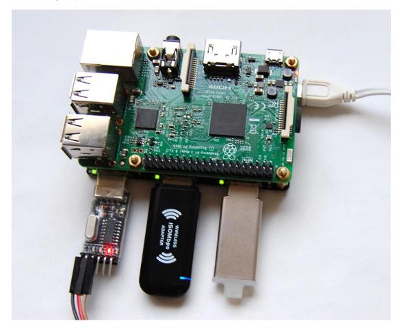
If you don't want to use the back-powering, just take out the pogo pins from their holders. After doing so, you will need two power supplies, one for the USB hub and the other for Raspberry Pi. You will need a mini-USB cable for connecting the USB hub to your Raspberry Pi. Also the jumper should be placed to the opposite side against "power link".
