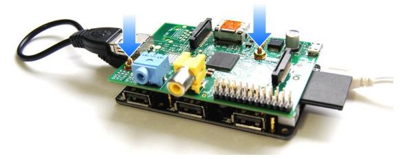
Use the USB - mini USB cable to connect the USB port on Raspberry Pi and the mini USB port on the USB hub and then it will be ready to work.
