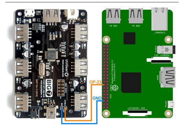
Usually the USB devices will get back to work after the power is resumed. However, sometime the USB hub may need a reset to make sure all connected USB devices will work properly.
