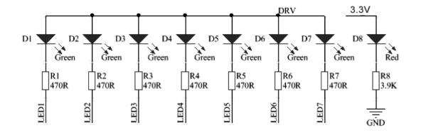
The green (or yellow) LED (D1~D7) will indicate if the corresponding USB port is currently being used, while the red LED (D8) is working as power indicator.
