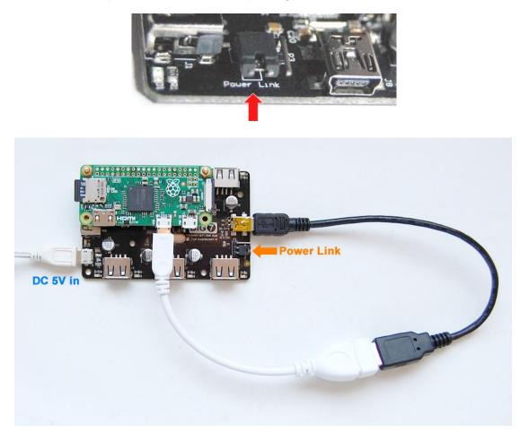
If you don't want the back-powering, just put the jumper to the other side and connect two power supplies to USB hub and Raspberry Pi Zero accordingly.
