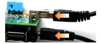
By default the jumper is at the "power link" position, and it can back-power your Raspberry Pi. When the power supply is connected to the USB hub, you will see your Raspberry Pi is getting powered too. This allows you to use only one power supply to
