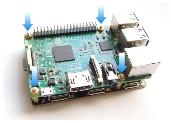
Raspberry Pi B+ and Raspberry Pi 2/3 (B model) do not support back-powering via USB port. However, you can use two pogo pins (included in the package) to let the USB hub to back-power your Raspberry Pi via the (bottom of) 40-pin header.
