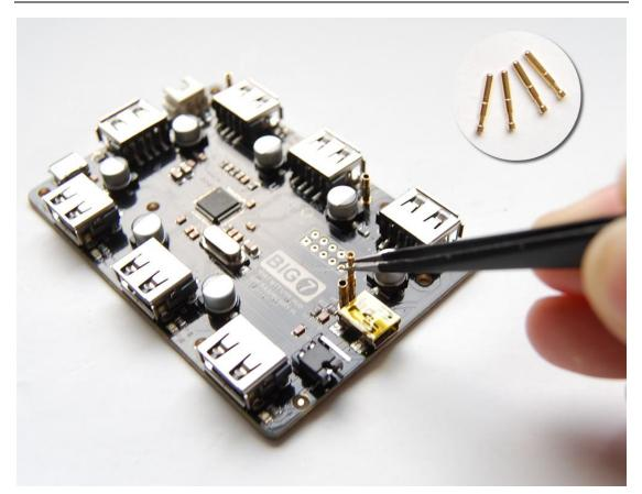
There are 4 pogo pin holders on the USB hub board. Gently put the pogo pin into the holder and press it to the bottom. You can use the other end of the tweezers.
