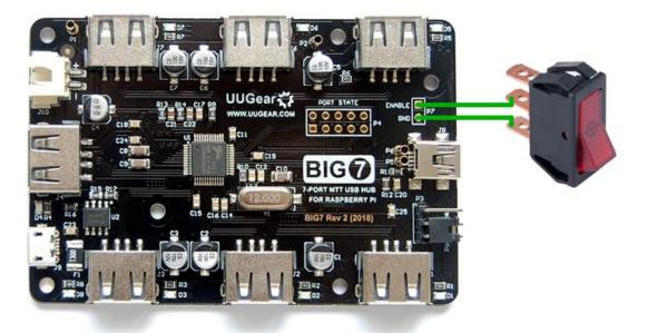
You can also connect the ENABLE pin to a GPIO pin in Raspberry Pi, and control the USB ports' power by setting the GPIO pin high/low.
