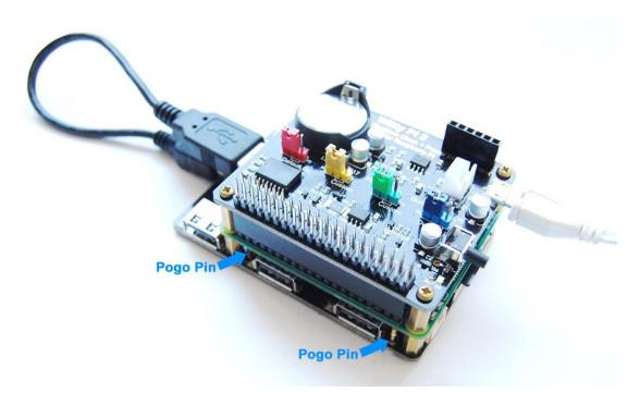
For Raspberry Pi A, B and compute module with development kit, Witty Pi 2 could not be mounted on them because of the incompatible GPIO pin header. Also they could not use the pogo pins to power the USB hub, so the USB hub can only work in bus-power mode. Having all these factors considered, it doesn't worth the effort to put them together.
