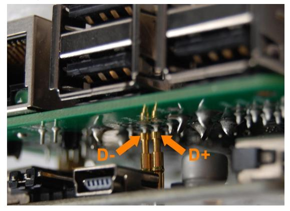
Although the pogo pin has cupped head, which is helpful for aligning to the joint point, it is still a challenge to align 4 of them a time. We found that following the steps below could make things easier:
