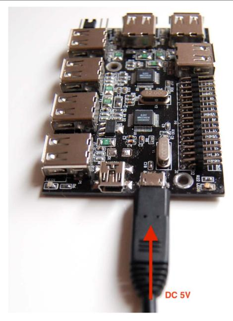
While using the self-power mode, you could choose to backfeed power to Raspberry Pi or not. By connecting the "Power Connection" jumper, Raspberry Pi could be powered by via the upstream USB port on the hub:
