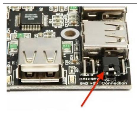
It is the recommended way to power the USB hub and Raspberry Pi with just one AC adapter. If you don't want the backfeed power, make sure to disconnect the "Power Connection" jumper, and then power the hub and Raspberry Pi separately:
