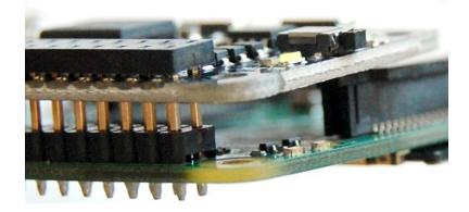
In order to make reliable connection, we suggest to use a <u>stacking pin header</u> (not included in the package).
