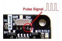
By default, the dummy load is off. If you turn the switch to the right side, the pulsing signal will be connected to a MOSFET, and controls the on/off of load (R20).
