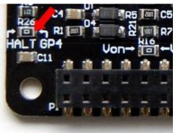
You will also need to modify the software a little bit to use different GPIO pins. More details here: <u>http://www.uugear.com/portfolio/change-the-pin-that-used-by-witty-pi/</u>
