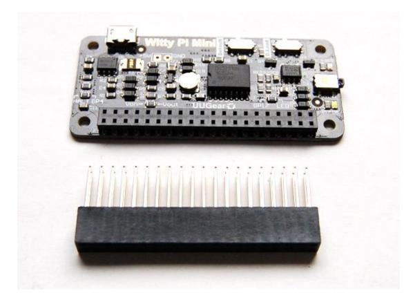
The 40 extra long pins on stacking header should reach the female header via the holes on the back of Witty Pi Mini. You can then place a steel ruler (or something
