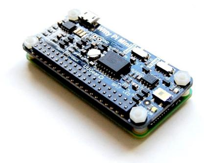
You will need to connect the power supply to the micro USB connector on Witty Pi Mini to make it work. Or you can power it via the (unpopulated) alternative power input connector.
