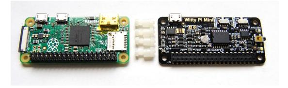
You can simply mount Witty Pi Mini on your Raspberry P Zero's 40-pin header, and it can work just like that. However, if you wish, you can use the plastic screws, spacers and nuts in the package to tightly mount Witty Pi Mini on your Raspberry Pi Zero. Please make sure NOT to put Witty Pi Mini up side down, the 40 pins should connect to the female header via the holes underneath, as shown in figure below.
