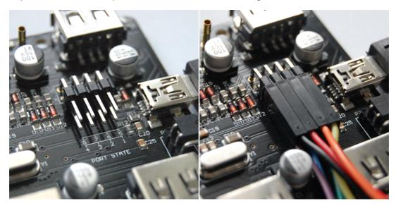
The figure below shows the layout of the pin header. The output pin is in HIGH voltage level when the corresponding USB port is not used. If you plug a USB device on a USB port, its port activity LED (green) will light up and its digital output pin will turn to LOW voltage level.
