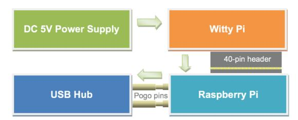
With this setup, the USB hub will work in self-power mode, which maximizes the output current of all USB ports.
