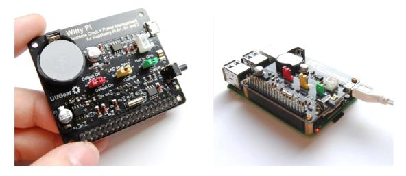
Since this USB hub can be mounted under Raspberry Pi, it has no conflict with Witty Pi. Instead it can be easily integrated into the Witty Pi + Raspberry Pi combination and become a nice sandwich structure.
