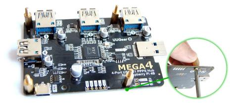
Then you can put your Raspberry Pi 4B on top, and secure it with the copper nuts.
