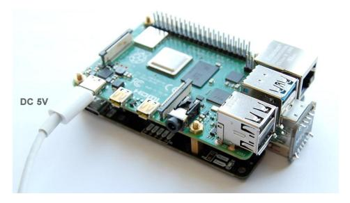
If you are going to connect some power hungry devices to MEGA4, it is better to connect another 5V power supply to MEGA4. This will significantly increase its ability of outputting high current.
