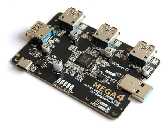
MEGA4 has the same board size as Raspberry Pi 4B, and can be mounted underneath. The U-shaped adapter (included) can make data and power connection between MEGA4 and Raspberry Pi.
