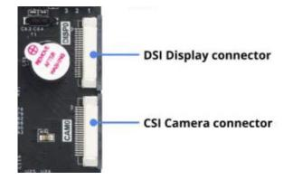
Different than the official Raspberry Pi Compute Module 4 I/O board, PiGear Nano uses I2C-1 instead of I2C-0 for DSI and CSI.
