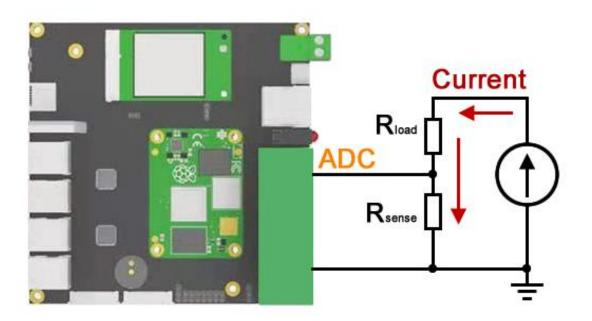
Usually  $R_{sense}$  is a rather small resistor. If  $R_{sense}$  is 0.01  $\Omega$ , and the voltage drops on  $R_{sense}$  is 0.0125V, the current can be calculated like this:
