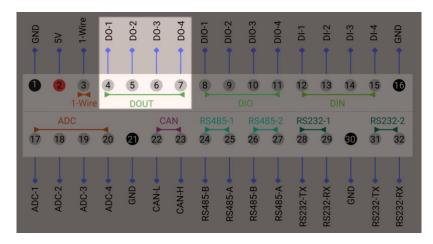
These 4 digital outputs are open drain outputs and they are driven by GPIO-11, GPIO-16, GPIO-17 and GPIO-22 in Raspberry Pi Compute Module 4 (please see table below).
