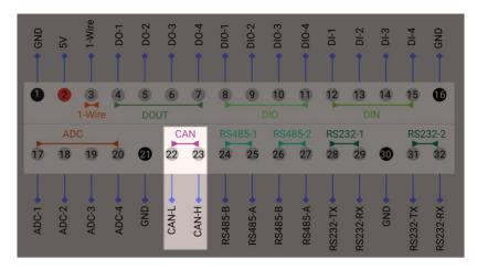
PiGear Nano uses chip MCP2515 to provide CAN controller, which talks to Raspberry Pi Compute Module 4 via SPI interface.
