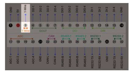
PiGear Nano uses chip DS2482 to implement a single-channel 1-wire master device, which talks to Raspberry Pi Compute Module 4 via the I2C-1 interface.
