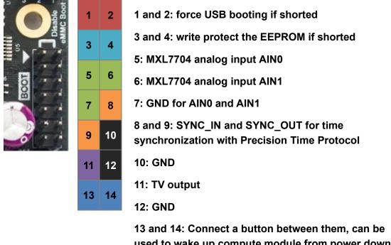
13 and 14: Connect a button between them, can be used to wake up compute module from power down. Has no effect when Raspberry Pi CM4 is on.
