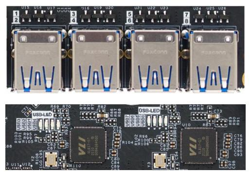
Limited by Raspberry Pi CM4's PCI Express Gen 2 lane, these 8 USB 3.0 ports share a total of 4Gbps of data bandwidth. However, there are scenarios that need to connect multiple USB 3.0 devices at the same time, while they don't have to work simultaneously. Providing 8 USB 3.0 ports indeed unlock many possibilities and offers more flexibility.
