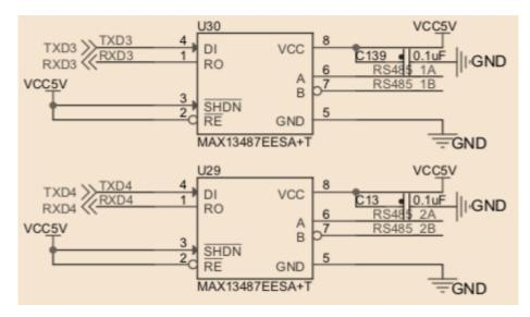
Both RS485 channels work in Half-Duplex mode, and they do not need additional I/O pin to control the transmitting direction.
