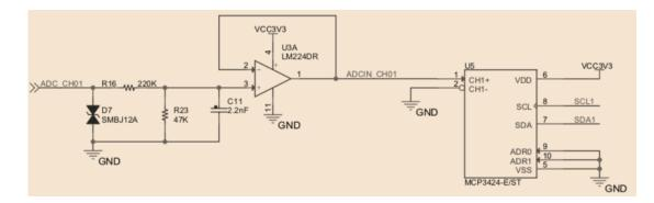
As shown in the schematic above, each channel has a voltage divider and a voltage follower before feeding to MCP3424. Because MCP3424 uses 2.048V internal voltage reference, each channel can directly measure up to 11.6V.
