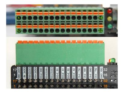
On the back of the board, you will also see the silkscreens that mark the functionality of each pin. Remarks: the silkscreen has the same layout as the soldering pads (instead of the holes on the connector), please pay attention to those numbers aside.
