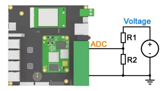
R1 and R2 should be properly chose so the actual voltage applies to ADC is no higher than 11.6V. In this case, the formula is changed to:
