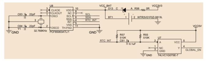
PCF85063 has very small quiescent current  $(0.22\mu A)$  and PiGear Nano uses a 3V 1F supper capacitor (BT1) for off-power time keeping. There is no need to use battery to keep the system time when the board is not powered.
