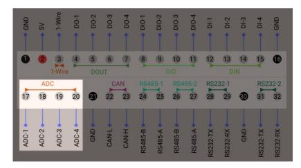
PiGear Nano uses chip MCP3424 to provide four-channel, low-noise, high accuracy A/D converter with up to 18-bit resolution. The A/D converter talks to Raspberry Pi Compute Module 4 via the I2C-6 interface.
