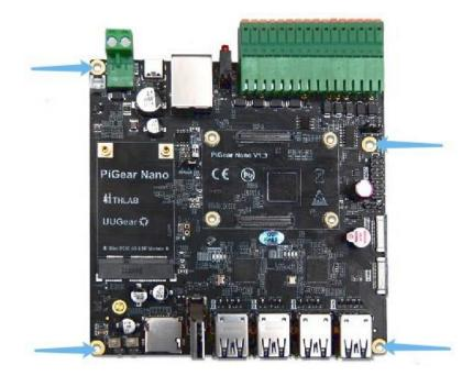
Connect Raspberry Pi Compute Module 4 to the board by simply aligning it with the two connectors on board (or alternatively you can align the CE marks on CM4 and the board), and then give it a good squeeze. It will crunch into place (and you can hear it).
