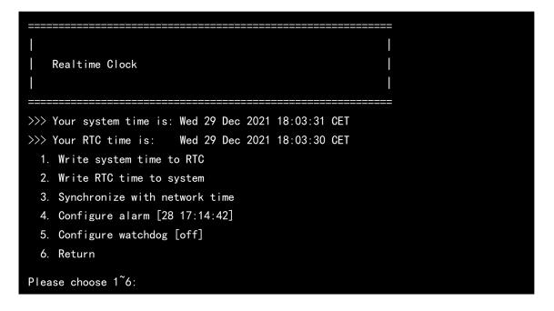
The real-time clock has one alarm and you can configure it to do different things. If you set the alarm time to a moment in the future (using option 4), the system will reboot when the alarm is triggered. If you do not use the e-latch power switch, which means your board will not be fully power off after shutdown, this alarm can also be used to wake up your Raspberry Pi.
