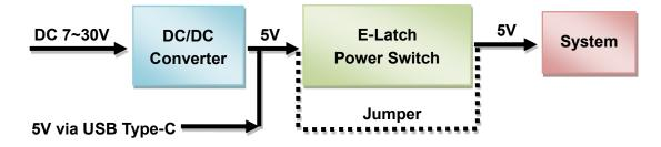
Our software installation script will enable the e-latch power switch support for you, however you will still need to <u>set the jumper</u> correctly to make it work.
