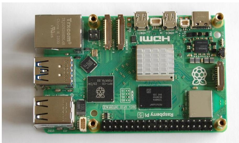
Next, mount Witty Pi 5's stacking header onto the 2x20 pin GPIO header of the Raspberry Pi and fasten it with the screws.
