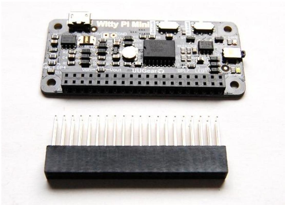
The 40 extra long pins on stacking header should reach the female header via the holes on the back of Witty Pi Mini. You can then place a steel ruler (or something
