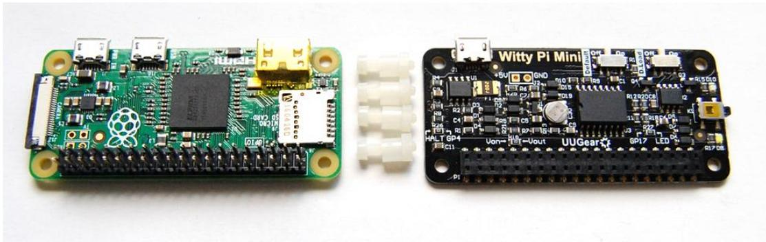
You can simply mount Witty Pi Mini on your Raspberry P Zero's 40-pin header, and it can work just like that. However, if you wish, you can use the plastic screws, spacers and nuts in the package to tightly mount Witty Pi Mini on your Raspberry Pi Zero. Please make sure NOT to put Witty Pi Mini up side down, the 40 pins should connect to the female header via the holes underneath, as shown in figure below.
