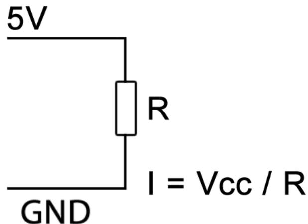
You can connect the resistor between the 5V and the ground, and you can make use of the unpopulated alternative power input connector.
