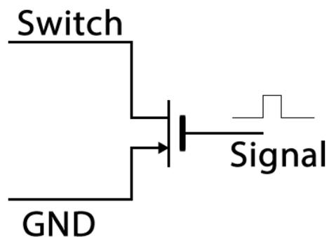
The signal should be a positive pulse, and the pulse length should be longer than 300ms. Processing a pulse will be equal to taping the switch once, so it will turn on your Raspberry Pi if your Pi is off, or turn off your Raspberry Pi if your Pi is on.
