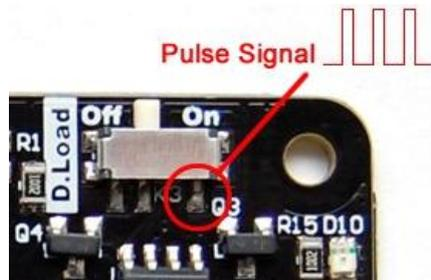
By default, the dummy load is off. If you turn the switch to the right side, the pulsing signal will be connected to a MOSFET, and controls the on/off of load (R20).
