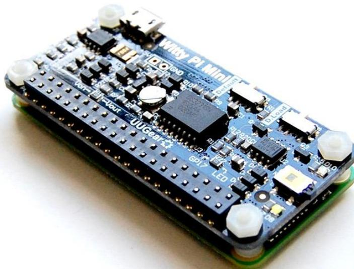
You will need to connect the power supply to the micro USB connector on Witty Pi Mini to make it work. Or you can power it via the (unpopulated) alternative power input connector.
