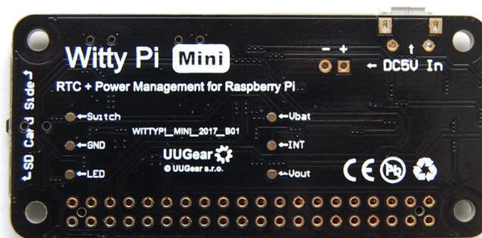
These testing pads were for product testing, but you can solder wires on them and them for extension and integration purpose.
