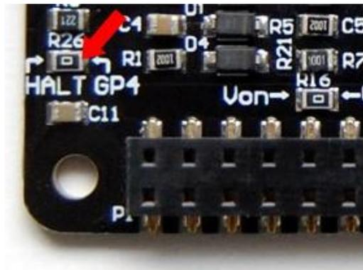
You will also need to modify the software a little bit to use different GPIO pins. More details here: <http://www.uugear.com/portfolio/change-the-pin-that-used-by-witty-pi/>
