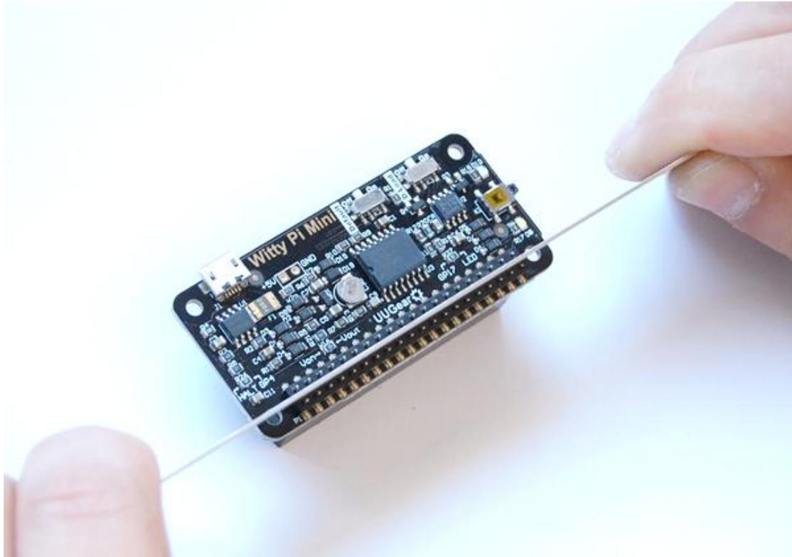
After mounting Witty Pi Mini on your Raspberry Pi, and connect the power supply to the micro USB connector on Witty Pi Mini, you can see **the white LED blinking, which means it is standing by.**
