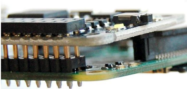
In order to make reliable connection, we suggest to use a [stacking pin header](#) (not included in the package).
