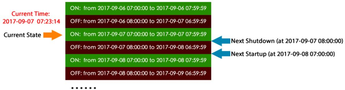
When the “runScript.sh” is executed, if the current time is located at an “OFF” state instead, it will take the next “ON” state as the current state, as it knows Raspberry Pi is currently ON.
